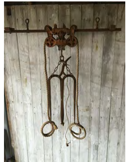
Hay Fork with Rope and Pulleys to Unload the Hay from the Wagon to the High Drive
